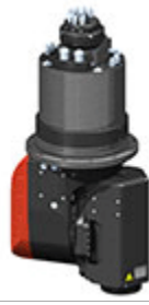
HST310D DIRECT DRIVE Rot. Axes A/C \pm 120^\circ/\pm 220^\circ//\pm 105^\circ/\pm 220^\circ -75kg~
